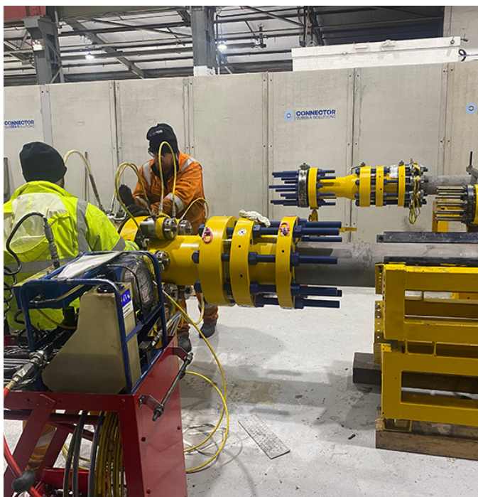
05 // MORGRIP® connectors tested in tandem.
