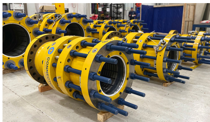
01 // CSS MORGRIP® Collet Connectors post factory acceptance testing.
