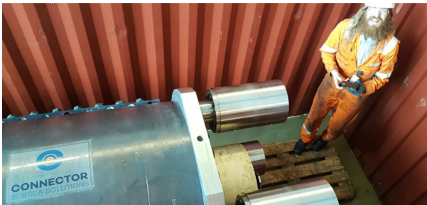
05 // CSS engineer carrying out pre-testing checks on the prototype clamp.
