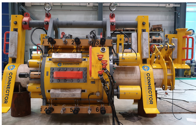
02 // CSS Holdback Clamp during factory acceptance testing (FAT).
