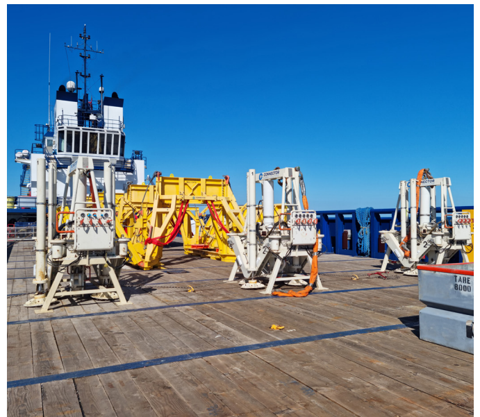
02 // CSS PLHFs and subsea mud mats unpacked and removed from shipping containers.
