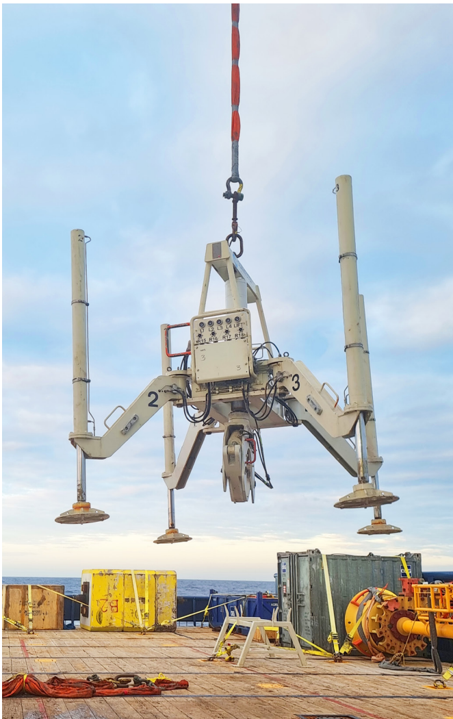
03 // CSS PLHF lifted for deployment.
