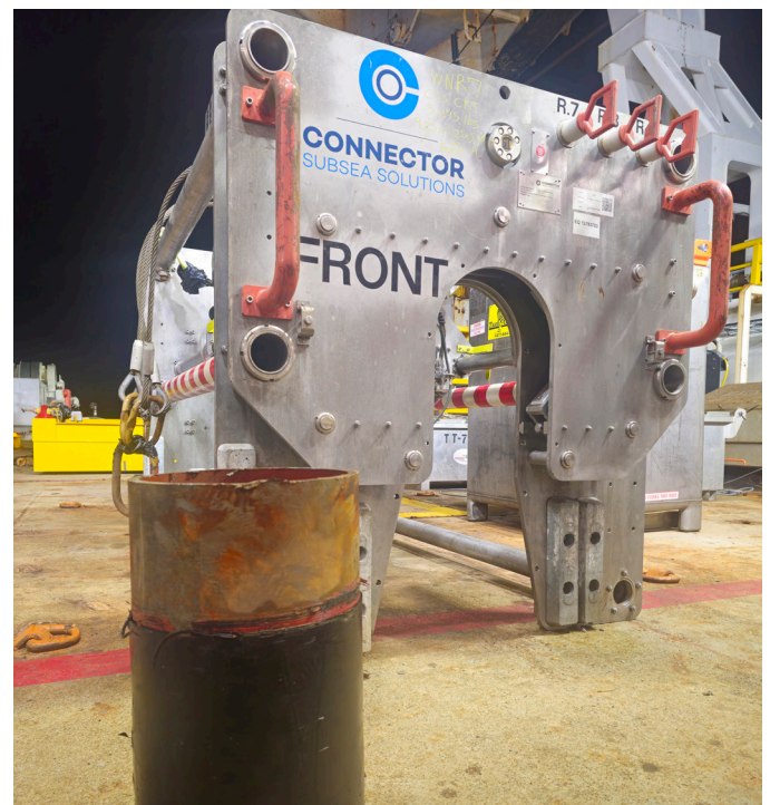
04 // CSS Deepwater CRT with a retrieved pipe section after coating removal.
