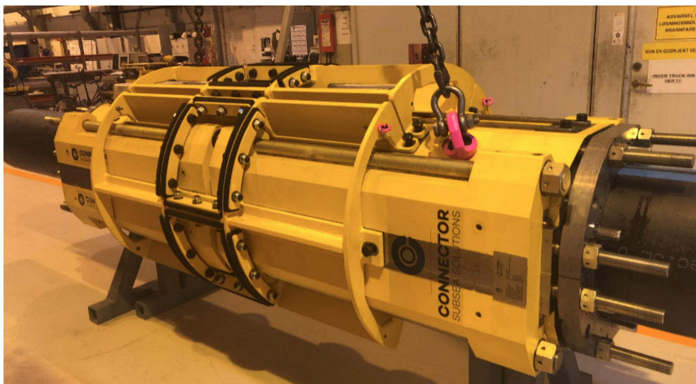
01 // The first-of-its-kind diver-friendly CSS MORGRIP® Conductor Repair Clamp
