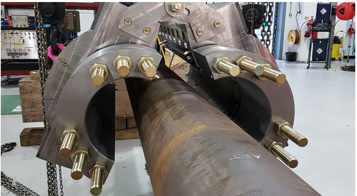
04 // Close-up of clamp closure over pipe during testing
