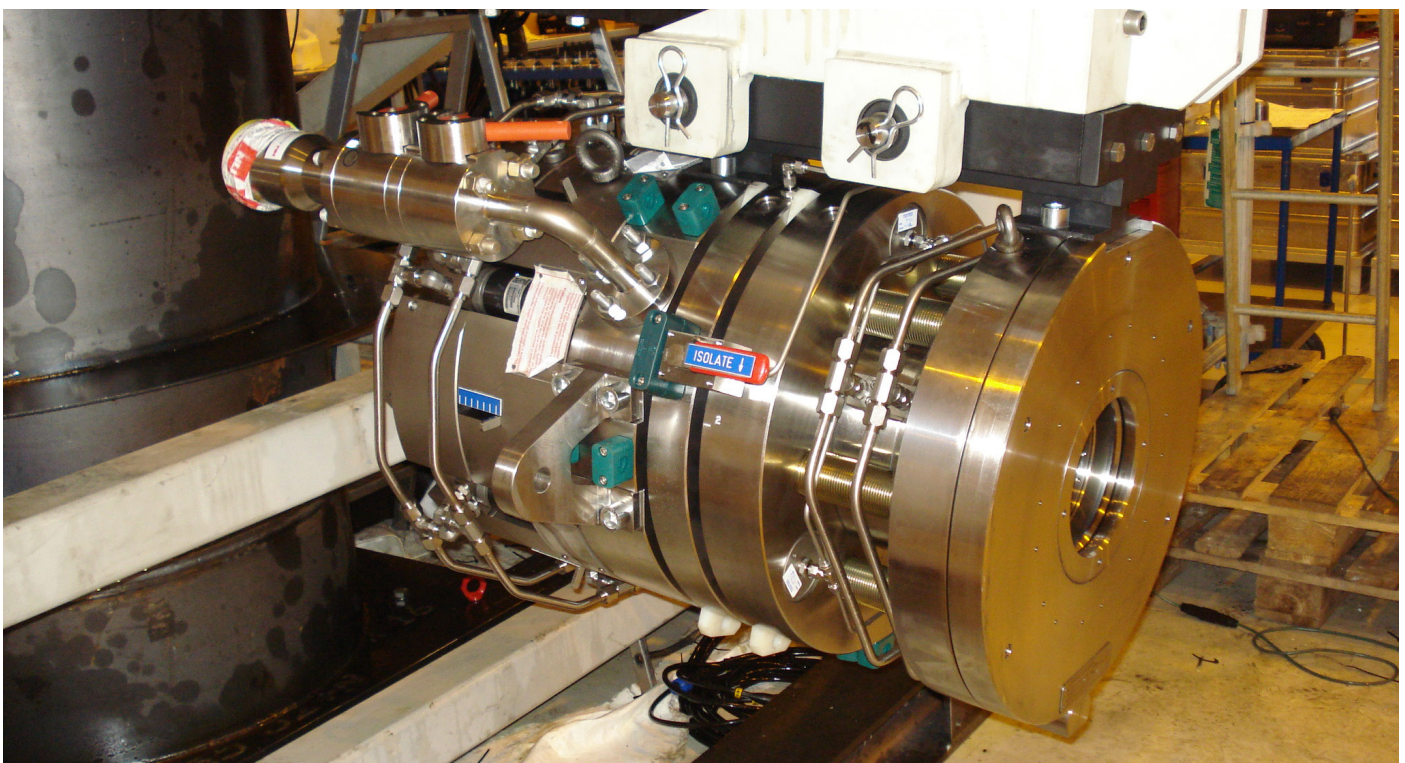
01 // MORGRIP® engineers created a special end-connector to handle a difficult repair
